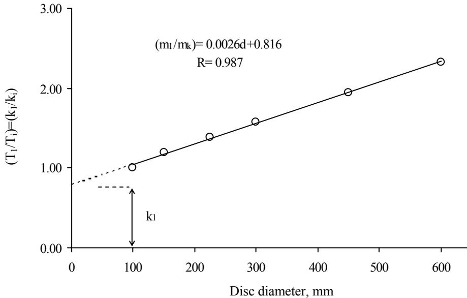
Figure 8. Linear relation between  $(T^1/T_i) = (k_1/k_i)$  and disc diameter.
