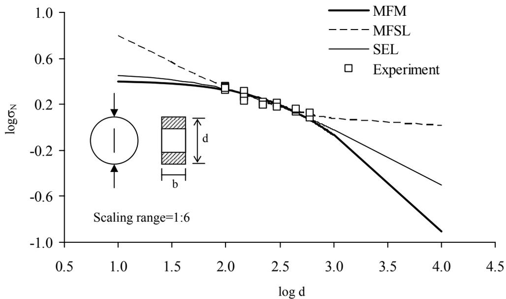
Figure 10. A typical comparison of MFM, MFSL, and SEL for  $2a/d=0.5$
