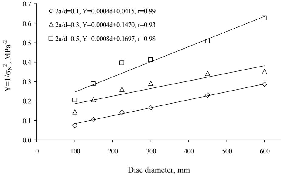
Figure 3. Linear regression results for notched concrete disc specimens obtained by Eser, 2002.
