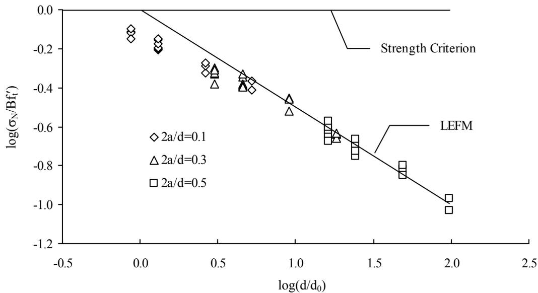
Figure 6. Test results of disc specimens obtained by Atahan, 1996 displaying the size effect.
