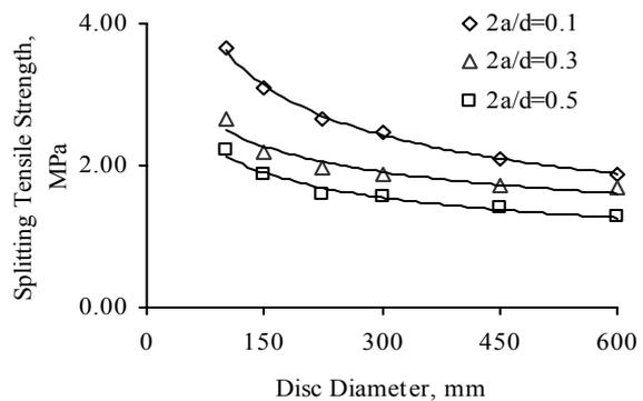
Figure 2. Relationship between the disc diameter and splitting tensile strength of concretes with notch.
