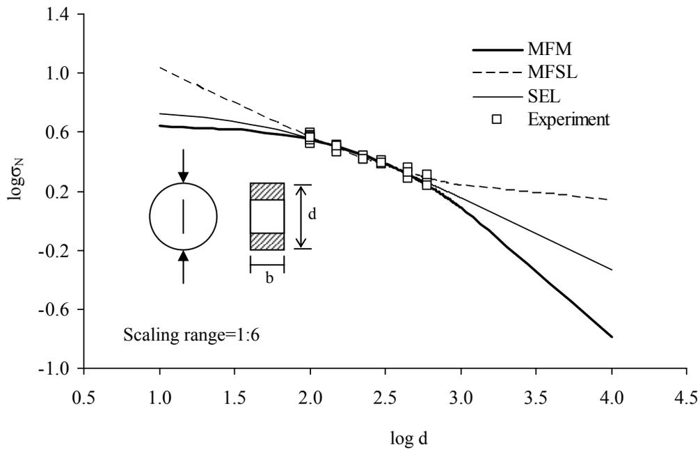
Figure 9. A typical comparison of MFM, MFSL, and SEL for  $2a/d=0.1$
