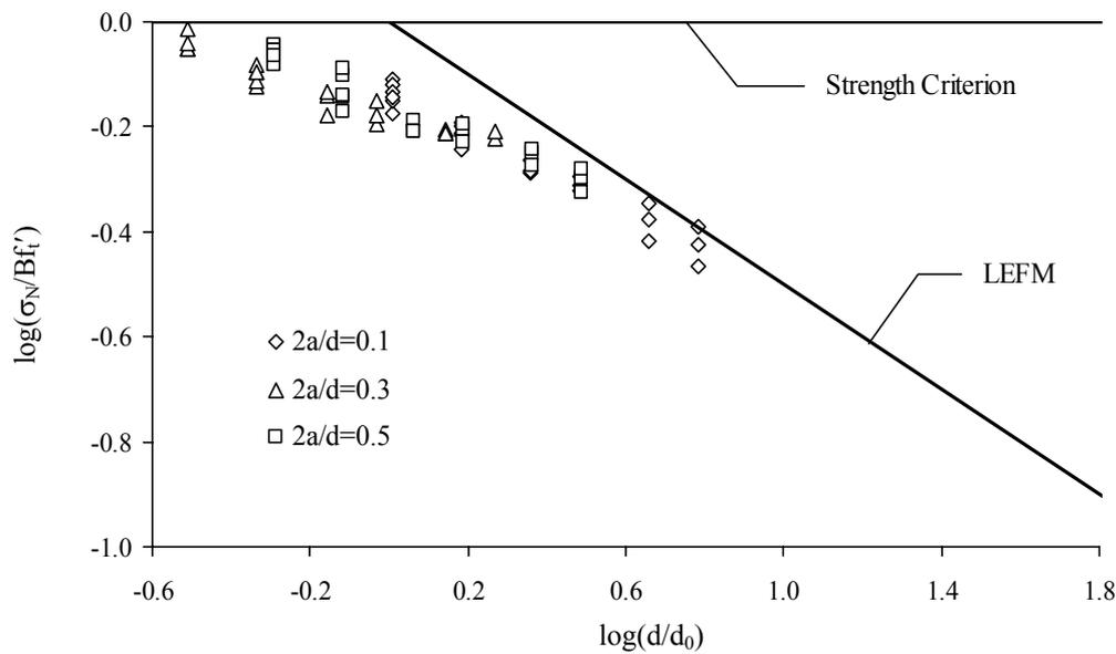
Figure 5. Test results of disc specimens obtained in this study displaying the size effect.
