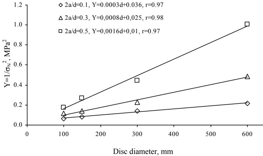
Figure 4. Linear regression results for notched concrete disc specimens obtained by Atahan, 1996.
