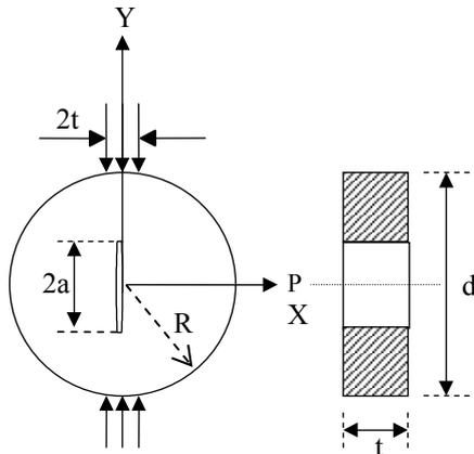
Figure 1. Loading setup condition and specimen geometry used in splitting-tensile tests.
