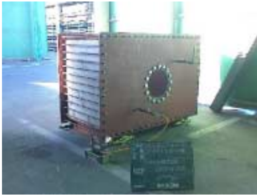
Figure 10. Set-up for internal water pressure tests
