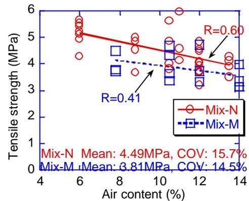
Figure 10. Effects of air content on tensile strength (TC test).
