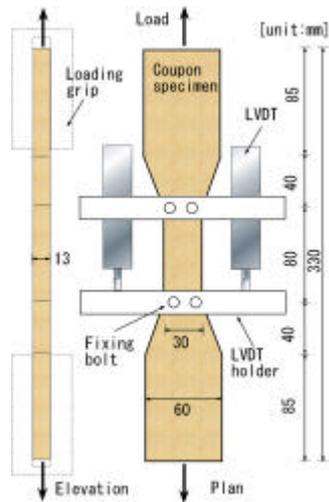
Figure 1. Tensile test of plate shaped specimen (TC test).
