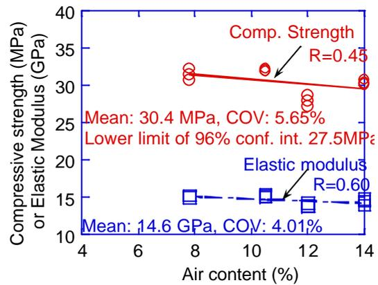
Figure 8. Effects of air content on mechanical performance (M-mix)
