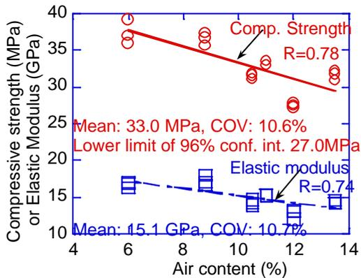
Figure 7. Effects of air content on mechanical performance (N-mix)
