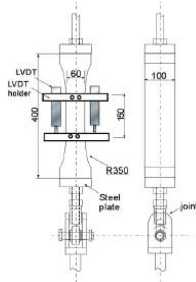
Figure 2. Tensile test of prism specimen (TP test).
