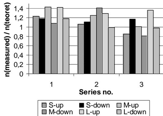
Figure 5. Measured versus theoretical (isotropic) number of fibres for series III: Beams made of vibrated concrete. S, M and L are the small, medium and large beams. The fibres are measured on the upper and lower half of the cross-section.
