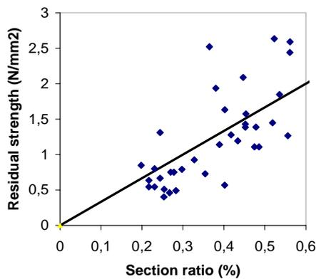
Figure 7. Residual strength versus measured section ratio for small beams (Series IV,  $b/h=150/150$ ).
