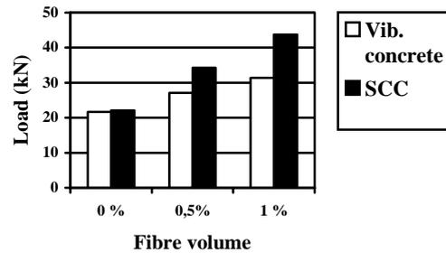
Figure 4. Moment capacity of beams made of ordinary and self compacting concrete with different steel fibre content. 60 mm long fibres with hooked ends
