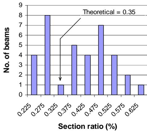
Figure 6. Section ratio for small beams (Series IV,  $b/h=150/150$ ), sawn out from real concrete structural elements.
