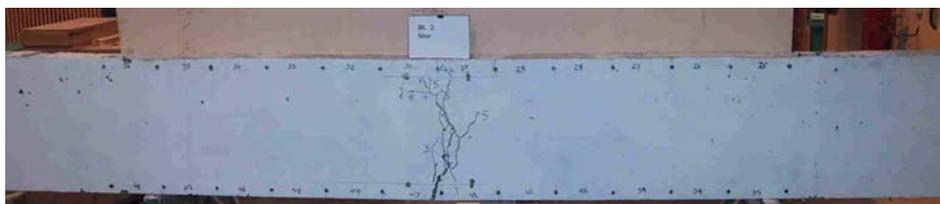
Figure 11. Crack patterns for the beams of series III. (a)  $h=150$ , 1% steel fibres and ordinary reinforcement, (b)  $h=250$ , 1% sf and ord reinf., (c)  $h=500$ , 1% sf and ord reinf, (d)  $h=150$ , 1% sf, (e)  $h=250$ , 1% sf, (f)  $h=500$ , 1% sf.
