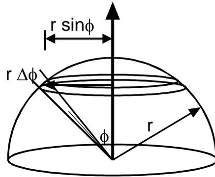
Figure 2. Determination of force resultant in the fibres crossing a crack. Thorenfeldt (2003).
