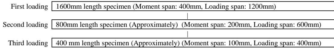
Figure 7. Experimental procedures (specimen length series)
