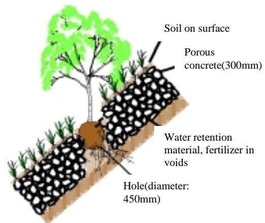
Figure 3. Image of porous concrete revetment (Tamai et al. 2003)
