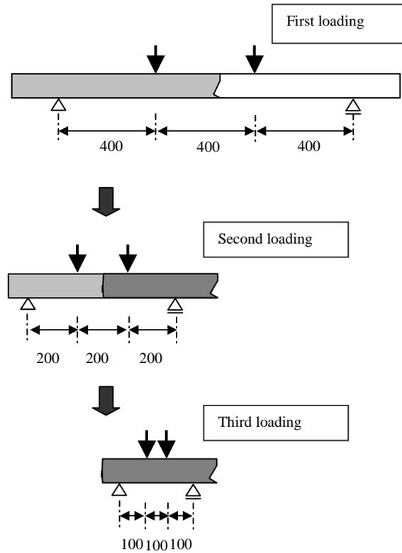
Figure 8. Test setup (specimen length series)
