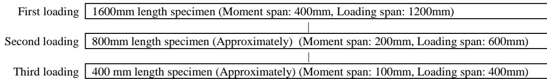
Figure 7. Experimental procedures (specimen length series)
