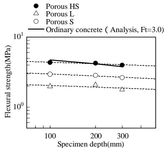
Figure 10. Flexural strength (specimen depth series)
