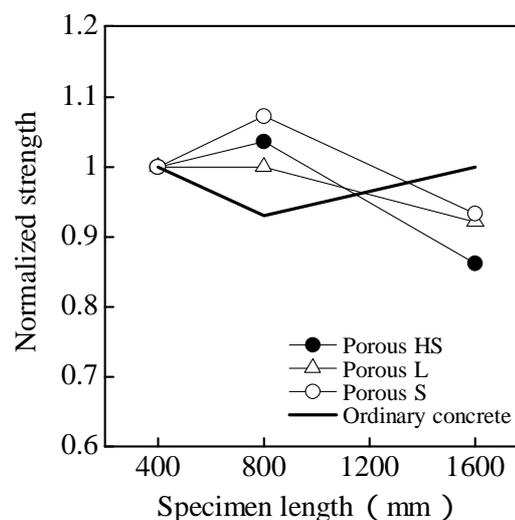
Figure 11. Flexural strength (specimen length series)
