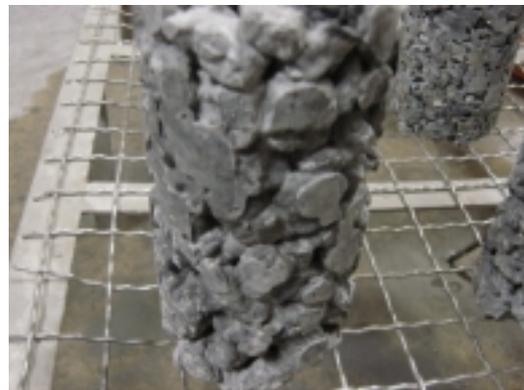
Figure 1. Porous concrete specimen (aggregate size: 13~20mm)
