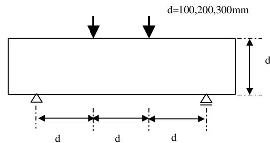
Figure 6. Test setup (specimen depth series)
