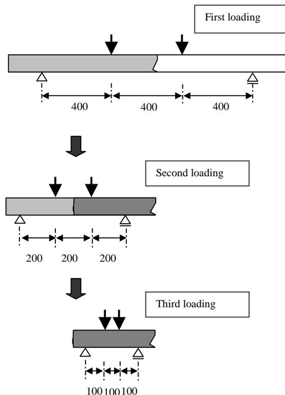
Figure 8. Test setup (specimen length series)
