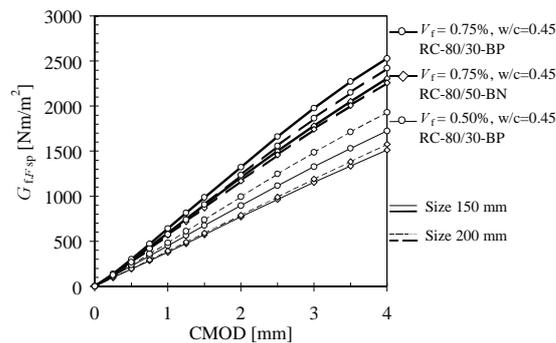
Figure 19. Comparison of the fracture energy evaluated from the two specimen sizes. For specimens from Mix 3 to 6, dashed line indicates the specimens with a size of 200 mm.
