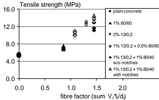
Fig. 4: Tensile strengths for different types of Hybrid-Fibre Concrete
