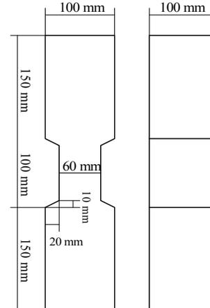
Figure 2 Shape and dimension of tensile specimen
