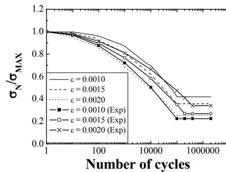
Figure 6 Comparison between bridging stress degradation relation obtained by experiment and micromechanics based model
