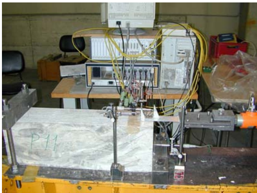
Figure 1: (a) Geometrical characteristics of FRP – concrete specimens, scheme and (b) picture of experimental setup.
