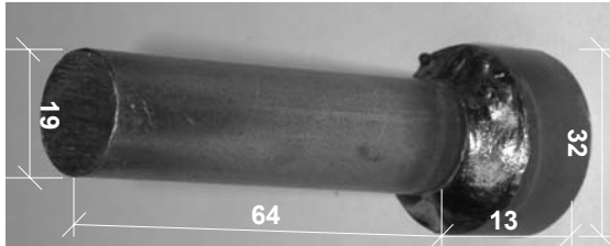
Figure 3. Geometry of a shear stud (unit: mm)
