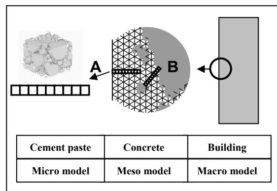
Figure 1. Schematic representation of micro- meso- and macro-level modelling.
