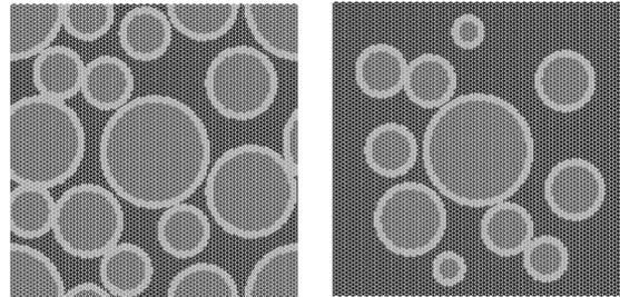
Figure 6. Lattice meshes used; periodic boundary lattice (left), free boundaries (right).
