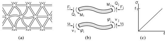
Figure 5. Lattice of beam elements (a), definition of forces and degrees of freedom (b), stress-strain relation of beam element (c).
