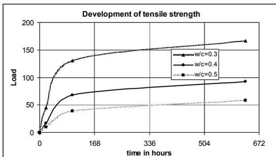
Figure 10. Development of tensile strength in time for 3 mixes.
