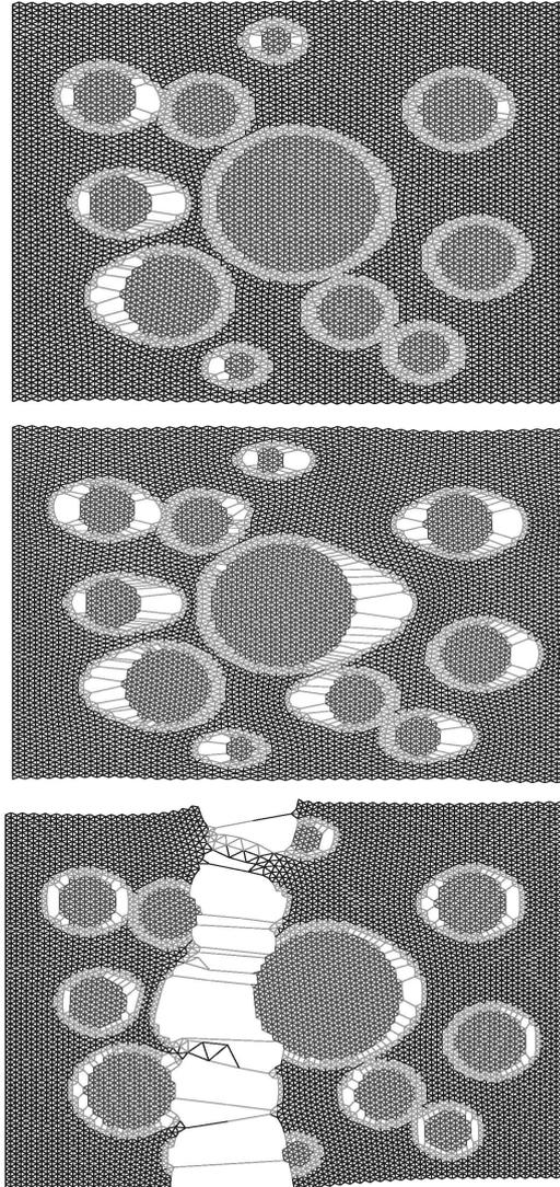
Figure 9. Simulation of tensile fracture; pre-peak (top) at peak load (middle); post-peak (bottom).
