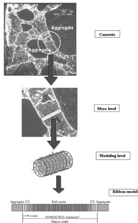
Figure 2. Overview of the ribbon model, (Koenders et al. 2003).
