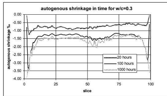
Figure 3. Autogenous shrinkage for mix with  $w/c=0.3$  at three stages of hydration: 20, 100 and 1000 hours.
