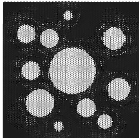
Figure 11. Eigenstresses in matrix after 20 hours of hydration;  $w/c=0.3$  (top),  $w/c=0.4$  (middle),  $w/c=0.5$  (bottom); light colors = tensile stress, dark colors = compressive stress.
