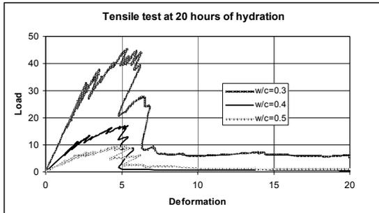
Figure 8. Load deformation curves in tension after 20 hours of hydration for 3 mixes.
