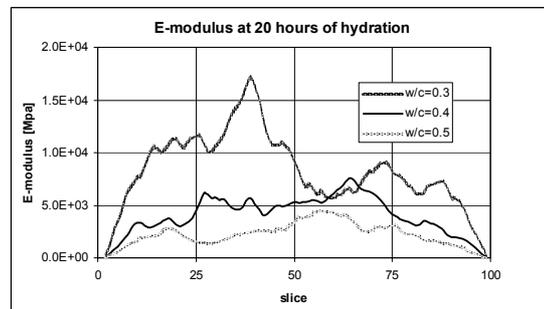
Figure 4. Autogenous shrinkage (top) and development of E-modulus (bottom) after 20 hours of hydration for three mixes, with different  $w/c$ .
