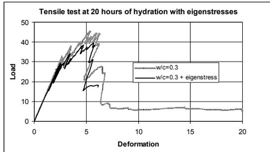
Figure 12. Load deformation curves for tensile test with and without eigenstress for  $w/c=0.3$  after 20 hours of hydration.
