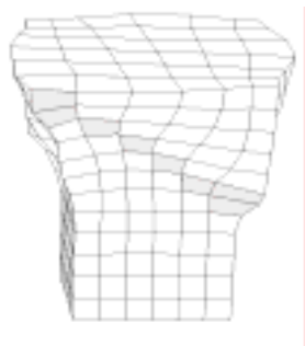
Figure 11. Shape of localized deformation during fracture.
