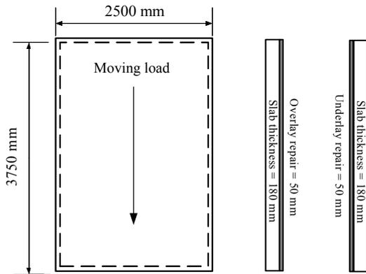
Figure 3. Dimension of overlay and underlay RC slabs
