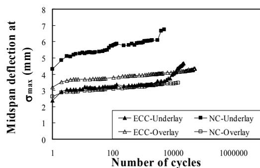
Figure 14. Comparison between midspan deflection of all repaired slab cases at fatigue load 480 kN
