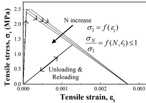
Figure 8. Stress-strain relationship of normal concrete under fatigue
