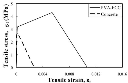
Figure 6. Tensile stress-strain relationships of cementitious materials
