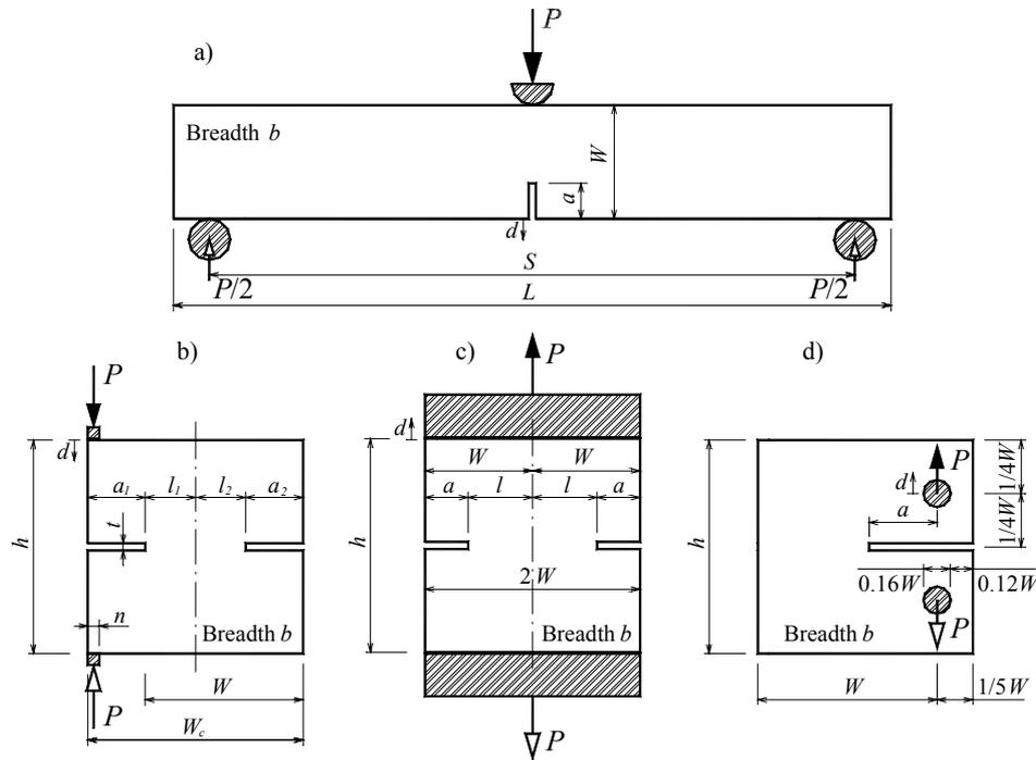
Figure 1. Testing configurations studied: a) SEN-TPB, b) DEN-EC, c) DEN-T and d) SEN-CT
