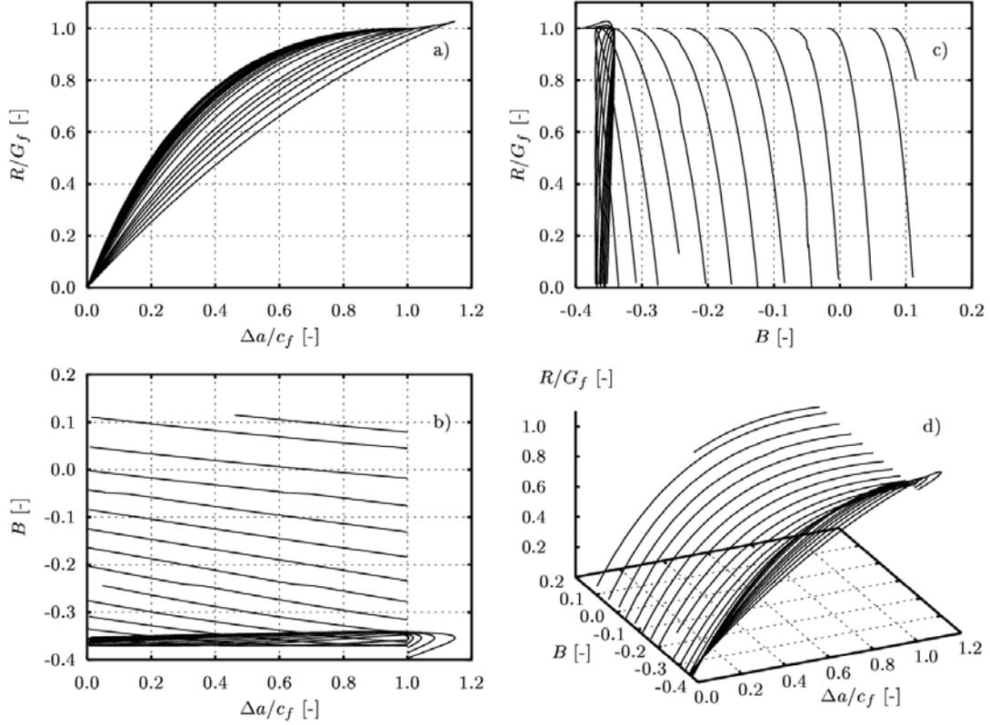
Figure 5.  $R$ -surface for DEN-EC configuration from  $R$ -curves for relative notch lengths 0.05, 0.06, 0.07, 0.08, 0.09, 0.1, 0.125, 0.15, 0.175, 0.2, 0.25, 0.3, 0.35, 0.4, 0.45, 0.5, 0.55, 0.6, 0.65, 0.7, 0.75, 0.8, 0.85 and 0.875 (from bottom to top in graph b)
