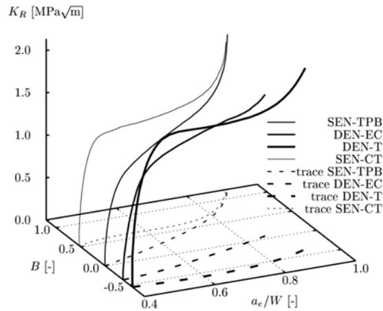
Figure 3.  $K_R$ -curves from compliance for testing configurations with different constraint of deformation near the elastic equivalent crack tip drawn into 3D plot
