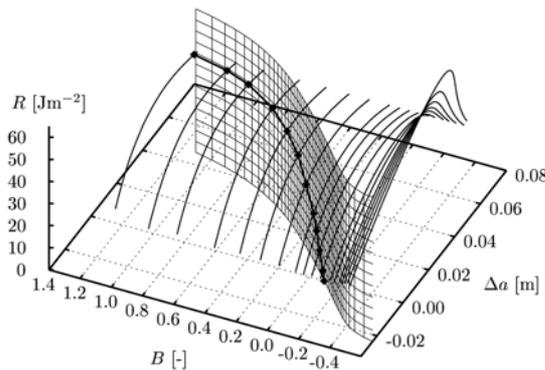
Figure 8. Extraction of "true"  $R$ -curve corresponding to specific case of geometry and size as an intersection of the  $R$ -surface with surface characterizing change of constraint of deformation during fracture (function  $B$ )
