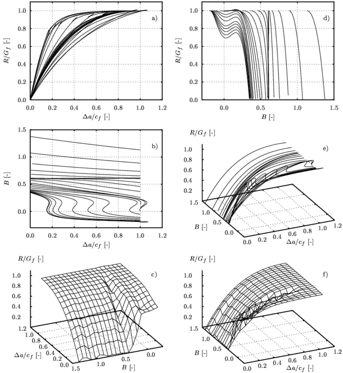
Figure 7.  $R$ -surface for SEN-CT configuration from  $R$ -curves for relative notch lengths 0.05, 0.055, 0.06, 0.065, 0.07, 0.08, 0.09, 0.1, 0.125, 0.15, 0.175, 0.2, 0.25, 0.3, 0.35, 0.4, 0.5, 0.6, 0.7, 0.75, 0.8, 0.85 and 0.9 (from bottom to top in graph b). An approximation of the surface is sketched in two views in graph c) and f)
