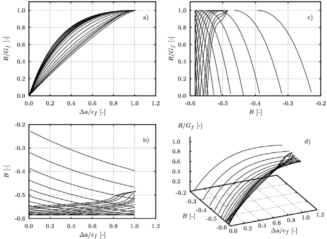
Figure 6.  $R$ -surface for DEN-T configuration from  $R$ -curves for relative notch lengths 0.06, 0.08, 0.1, 0.15, 0.2, 0.25, 0.3, 0.35, 0.4, 0.45, 0.5, 0.55, 0.6, 0.65, 0.7, 0.75, 0.8, 0.85 and 0.9 (from bottom to top in graph a)
