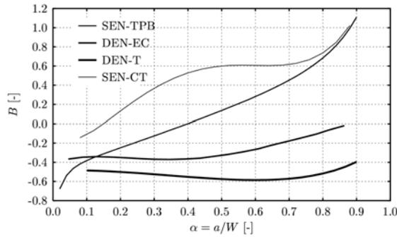
Figure 2. Biaxiality factor  $B$  as a function of relative crack length for analyzed geometries
