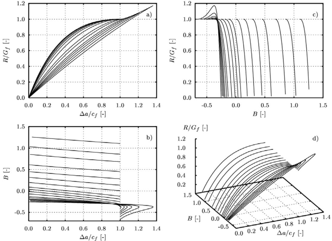
Figure 4. *R*-surface for SEN-TPB configuration constructed from size effect law *R*-curves for relative notch lengths 0.02, 0.03, 0.04, 0.05, 0.06, 0.08, 0.1, 0.15, 0.2, 0.25, 0.3, 0.4, 0.5, 0.6, 0.7, 0.8, 0.85 and 0.9 (from bottom to top in graph b)
