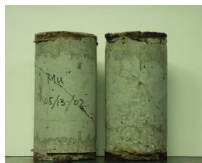
Figure 6. An inclined crack in the hollow cylinder specimens
