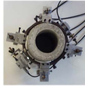
Figure 3. Experimental setup: LVDTs
