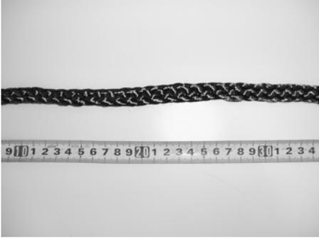
Figure 2. CFRP braiding.
