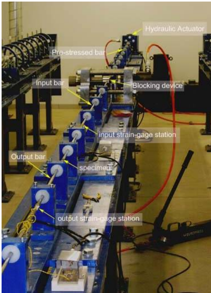
Figure 5. Set up for high strain-rate tests on steel specimens
