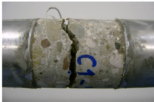
Figure 11. Large concrete specimen after failure
