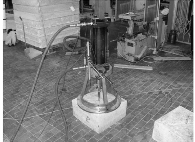
Figure 5. Loading rig during a typical pull-out test.
