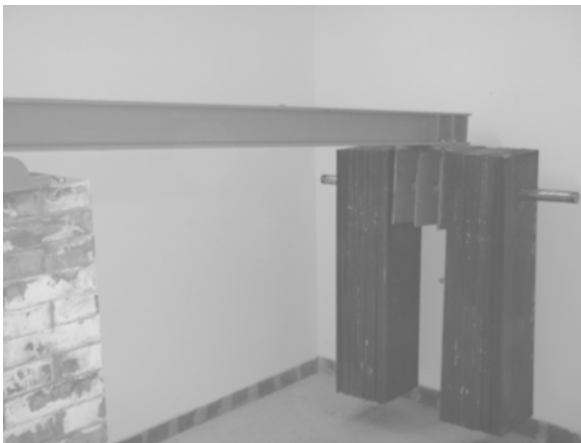
Figure 4. Dead loads applied by using steel sheets
