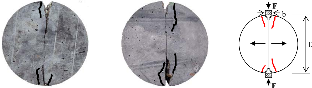
Figure 6. Fracture images of a high strength concrete with gravel aggregate (left, C100/115), high strength concrete with crushed aggregate (centre, C100/115) and schema of the fracture mechanism (right).
