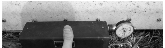
Figure 4. Measuring concrete surface displacements with a Whittemore gage.
