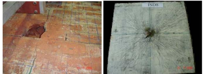
Figure 17. Impact and distal face of ISD8 after perforation.
