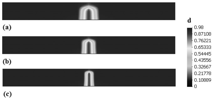
Figure 8. Local damage distribution in the beam: (a)- 300 elements, (b)- 600 elements and (c)- 1200 elements.
