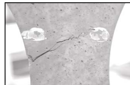
Figure 9. (a): Curves derived by the pendulum-bar tensile test with the specimen 0 0 3 C_II. (b): Crack pattern of the above mentioned specimen.
