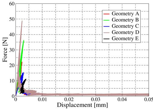
Figure 10: Typical Load-Displacement diagrams for 3D concrete prisms ( $P_k = 0\%$ , random lattice, 'medium') for case study IV, with the geometries A, B, C and D; see Figure 5
