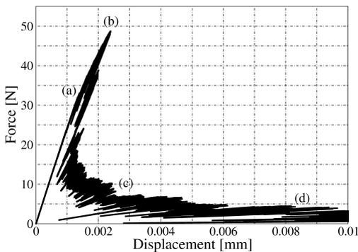
Figure 6: diagram from a 3D concrete prism analyzed with 122593 lattice elements (Table 2, size 'medium') and  $P_k = 35\%$ . The letters in brackets (a) - (d) show the transition points between the typical stages in the fracture process in concrete
