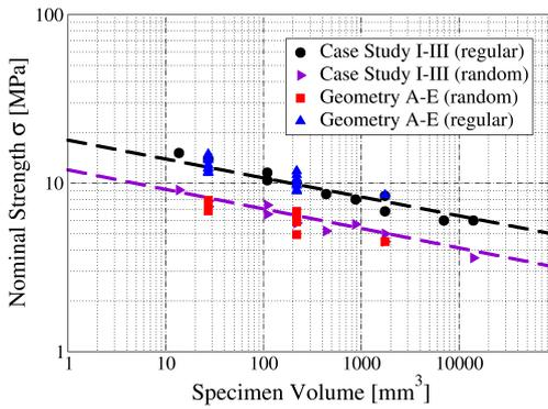
Figure 12: The present calculated nominal strength for the geometries A-E put on the same diagram on [Figure 9](#)
