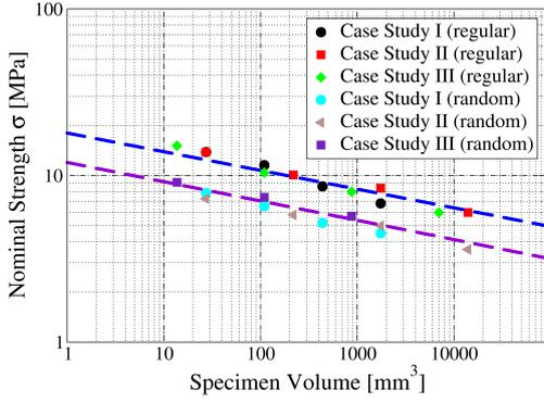
Figure 9:  $\log \sigma - \log V$  relationship for  $P_k = 0\%$  on a regular and random configuration
