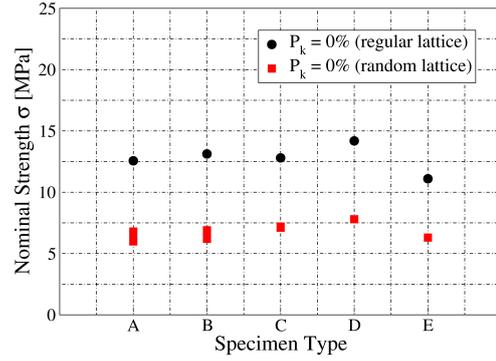
Figure 11: Comparison of the nominal strength for different shapes with identical volumes; case study IV (medium sized specimen)
