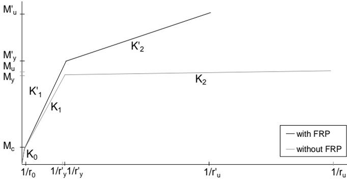
Figure 1: Moment-curvature diagram.
