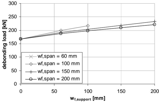
Figure 16: Influence of external reinforcement on the debonding mechanism: Anchorage failure (case B).
