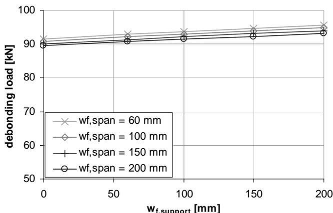
Figure 21: Influence of external reinforcement on the debonding mechanism: Concrete rip-off (case C).
