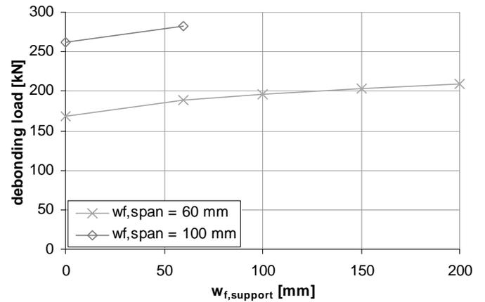
Figure 14: Influence of external reinforcement on the debonding mechanism: Debonding by force transfer (case C).
