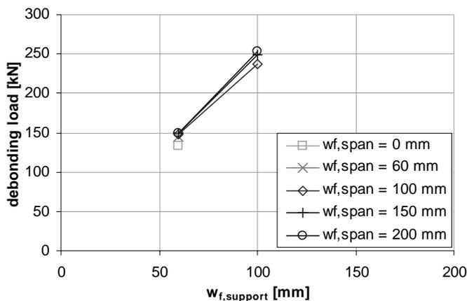
Figure 12: Influence of external reinforcement on the debonding mechanism: Debonding by force transfer (case A).
