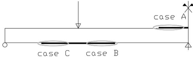
Figure 9: Differentiation between places of debonding.
