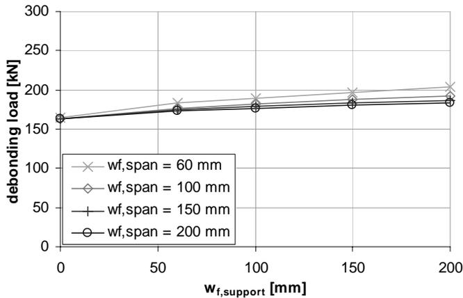
Figure 17: Influence of external reinforcement on the debonding mechanism: Anchorage failure (case C).
