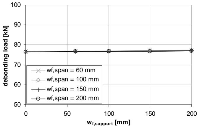
Figure 20: Influence of external reinforcement on the debonding mechanism: Concrete rip-off (case B).
