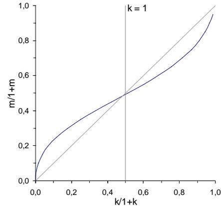
Figure 3: The relation of the moments  $m$  in function of the relation of the bending stiffnesses  $k$ .
