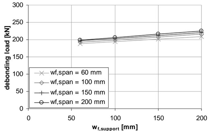
Figure 10: Influence of external reinforcement on the debonding mechanism: Debonding at cracks (case A).
