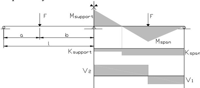
Figure 2: Continuous beam with variable bending stiffness (simplified to 2 stiffness zones).
