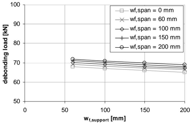
Figure 19: Influence of external reinforcement on the debonding mechanism: Concrete rip-off (case A).
