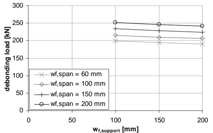
Figure 11: Influence of external reinforcement on the debonding mechanism: Debonding at cracks (case B).
