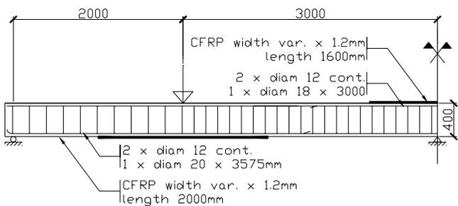
Figure 7: Internal and external reinforcement configuration.
