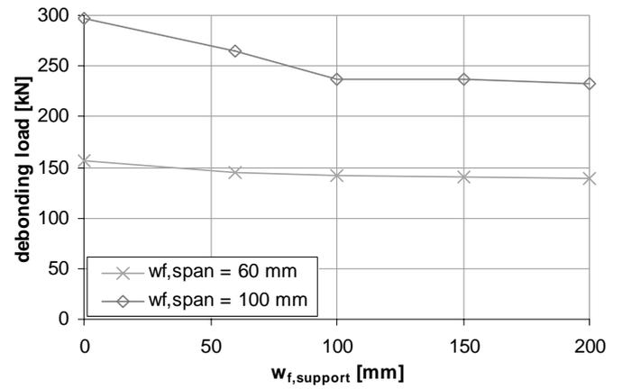
Figure 13: Influence of external reinforcement on the debonding mechanism: Debonding by force transfer (case B).
