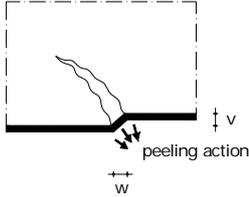
Figure 4: Peeling-off caused at shear cracks.
