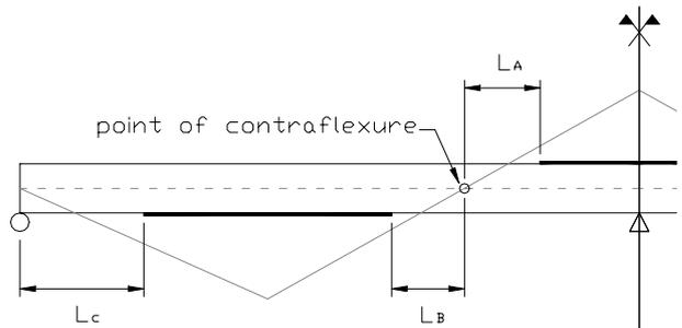
Figure 18: The distance  $L$  between the laminate end and the point where the internal moment equals zero.
