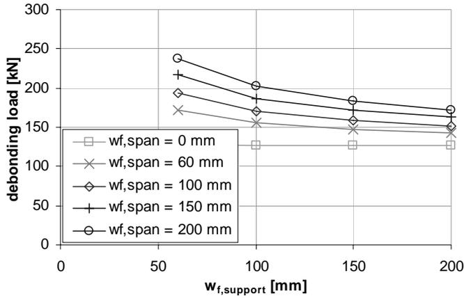
Figure 15: Influence of external reinforcement on the debonding mechanism: Anchorage failure (case A).
