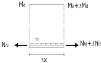
Figure 5: Peeling-off caused by force transfer.
