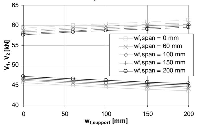
Figure 8: Shear force  $V_1$  in function of width of laminates.
