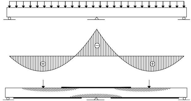
Figure 6: Moments with opposite signs in continuous beams and anchoring laminates into compression zones.
