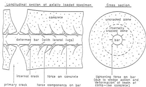
Figure 1. Internal cracks around the reinforcing bar embedded in concrete (Goto, 1971).
