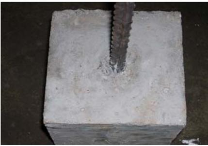
Figure 6. Pullout failure in confined concrete specimen.
