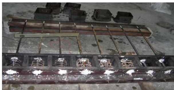
Figure 3. Confining reinforcement in pull-out specimens.
