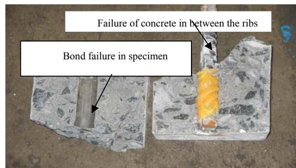
Figure 5. Splitting failure in unconfined specimen.
