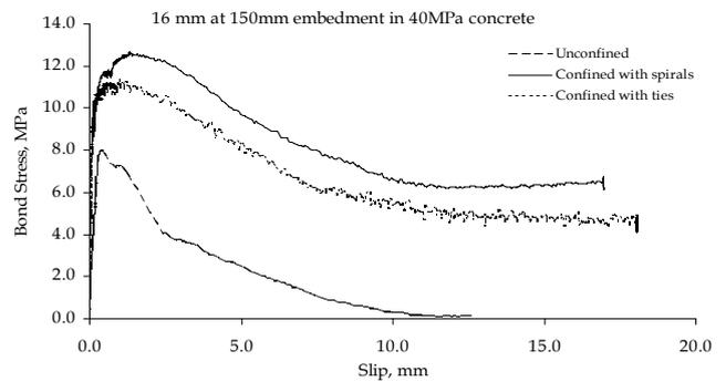
Figure 7. Bond stress vs. Slip with 16mm bars at 150mm embedment in 40 MPa concrete.
