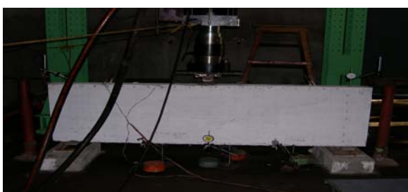
Figure 2. Beam specimen and experimental set up.
