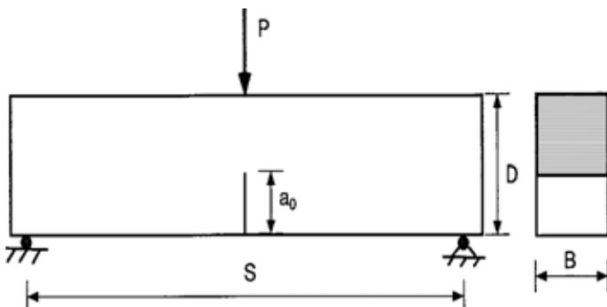
Figure 1. Configuration of a three-point bending notched beam
