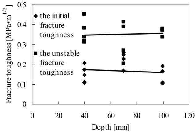
Figure 8. Influence of specimen depth on fracture toughness of cement paste
