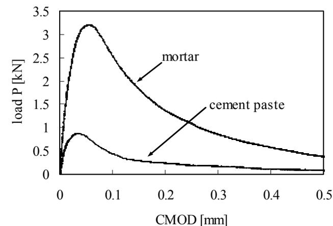
Figure 4. *P-CMOD* curves of different materials
