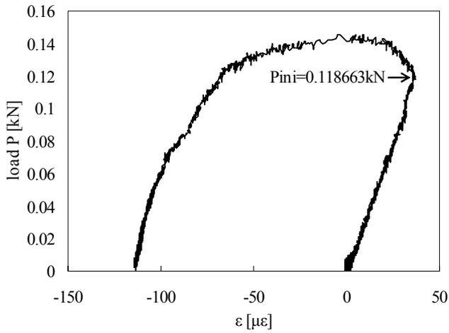
Figure 3. Determination of the initial cracking load
