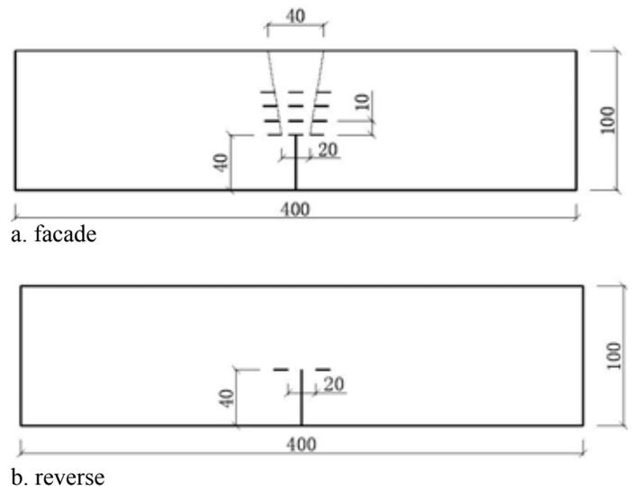
Figure 2. Arrangement diagram of the strain gauges
