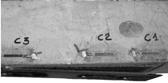
Figure 12: Photo of a failed beam due to FRP delamination.
