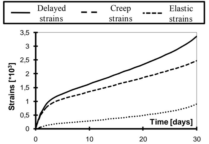
Figure 10. Contribution of “real” creep and elastic strains to delayed strains ( $\beta = 0.24$ , Eq. 4).
