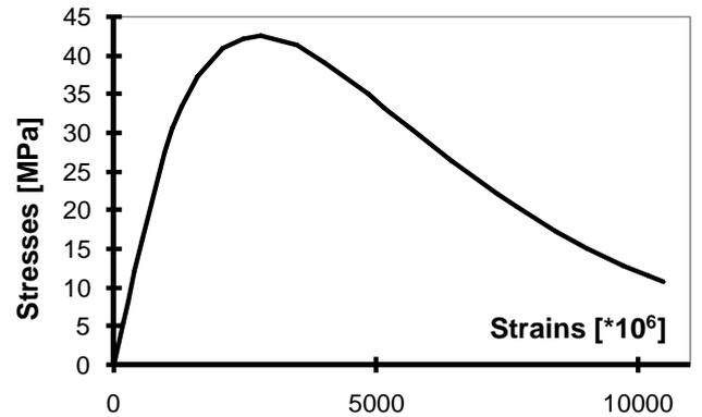
Figure 4. Stress – strain relationship in compression ( $\beta = 0$ , Eq. 4).
