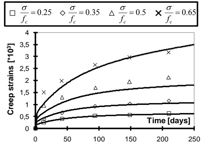
Figure 7. Delayed strains evolutions for different stress to strength ratios ( $\beta = 0.24$ , Eq. 4) – (experimental results from Roll, 1964).
