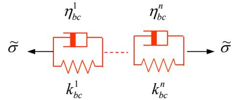
Figure 1. Kelvin-Voigt elements for the prediction of creep strains.
