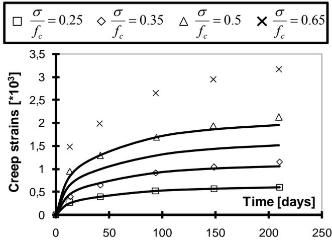
Figure 6. Delayed evolutions for different stress to strength ratios without taking into account creep/cracking interaction ( $\beta = 0$ , Eq. 4) – (experimental results from Roll, 1964).
