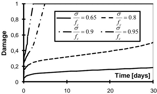
Figure 9. Damage evolutions with respect to time for different stress to strength ratios ( $\beta = 0.24$ , Eq. 4).
