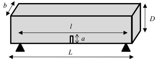
Figure 11. Geometry of the 3 points bending beam.
