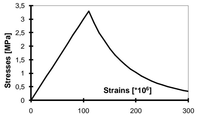
Figure 5. Stress – strain relationship in tension ( $\beta = 0$ , Eq. 4).
