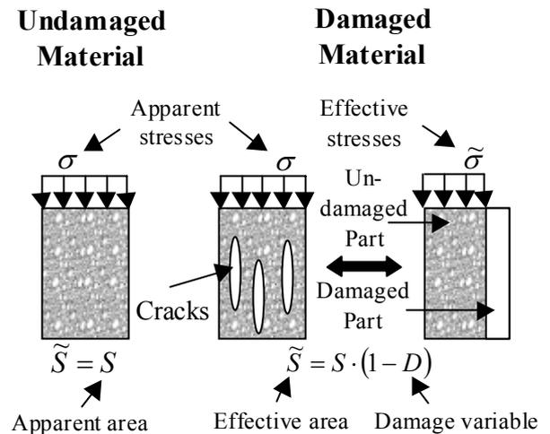
Figure 2. Definition of the damage variable.
