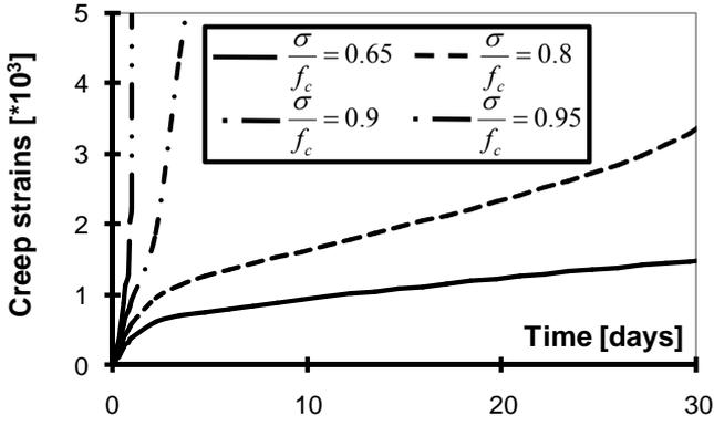
Figure 8. Delayed strains evolutions for different stress to strength ratios ( $\beta = 0.24$ , Eq. 4).
