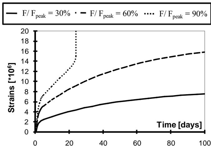
Figure 12. Delayed deflection with respect to time for different load to peak load ratios.
