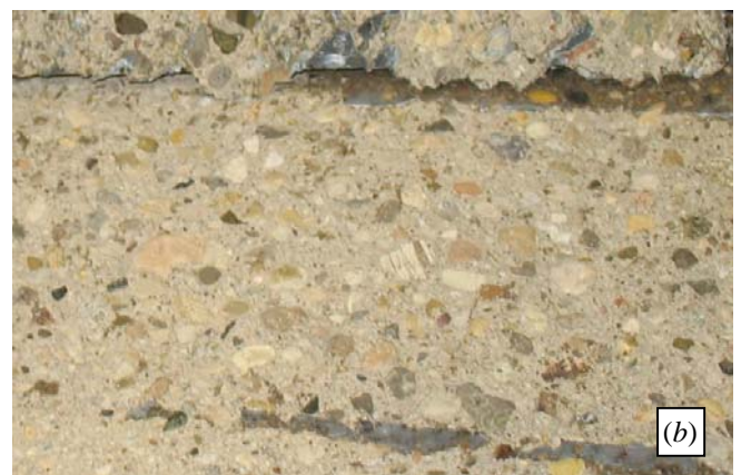
Figure 6. Fracture surfaces at the interface level of FRP – concrete specimens after debonding, with different surface preparations before adhesive application: (a) sand blasting and (b) grinding with a stone wheel with marble sand (type 1 grinding).
