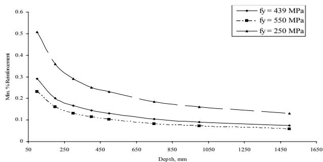
Figure 5. Min reinforcement vs. beam depth.
