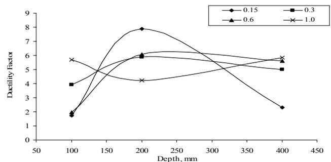
Figure 3. Ductility factor vs. beam depth.
