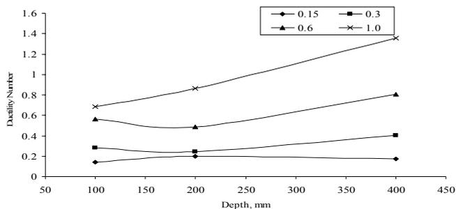
Figure 4. Ductility number vs. beam depth.
