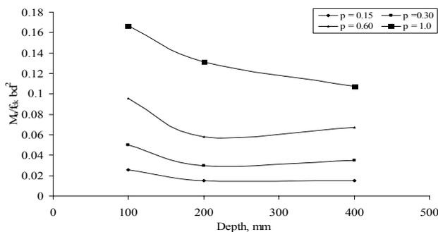
Figure 2. Moment ratio vs. Depth at different steel ratio.
