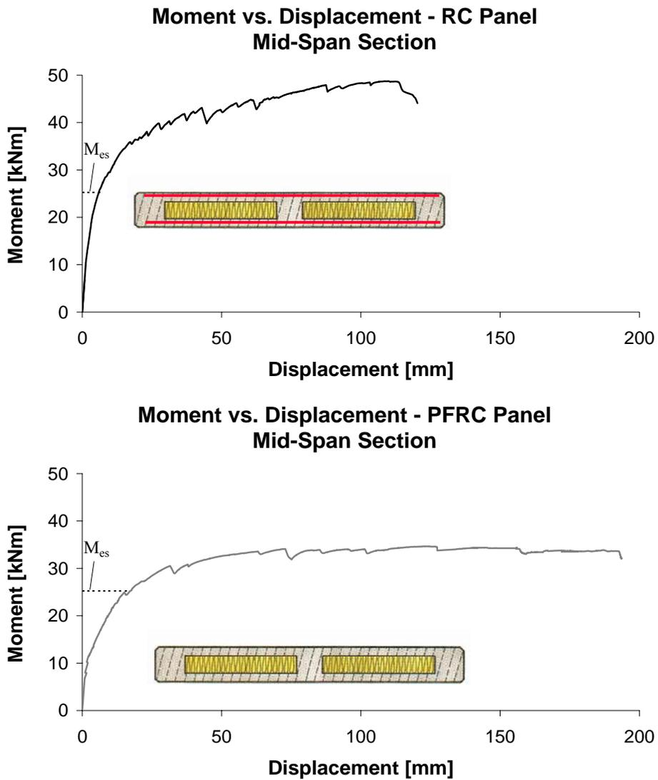
Figure 11. Comparison of the mid-span bending moment - deflection curves for the tested panels.
