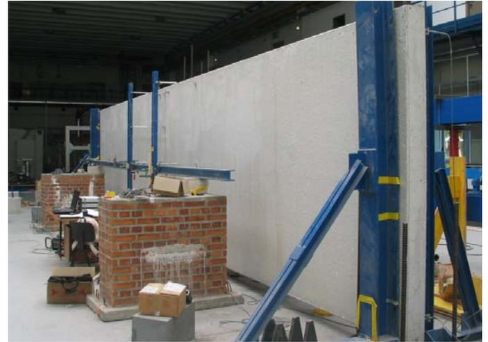
Figure 8. Panel placement on the reaction frame.
