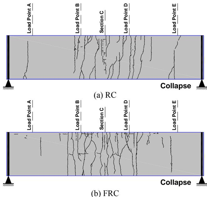
Figure 12. Comparison of the cracks distribution in the tested panels after the test.
