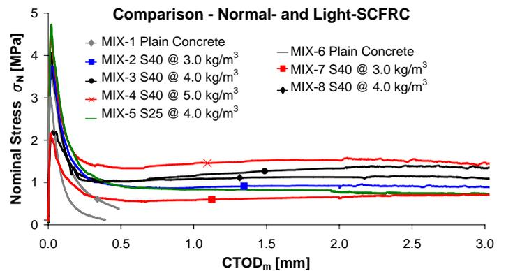
Figure 4. Comparison of the nominal stress versus CTOD curves (average curves) obtained from bending tests on both Normal SCFRC and Light-Weight SCFRC specimens.
