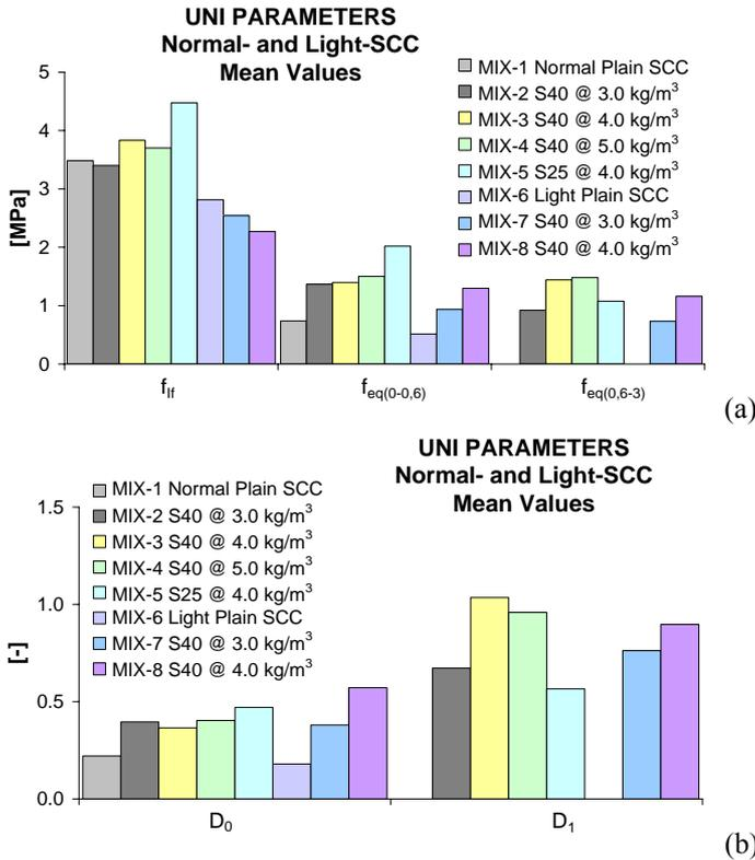
Figure 5. First-crack strength and post-cracking equivalent strengths (a) and ductility indexes (b) according to UNI 11039.
