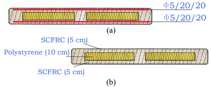
Figure 6. Geometrical characteristics of the transverse section of a traditional SCC panel (a) and a SCFRC panel (b).
