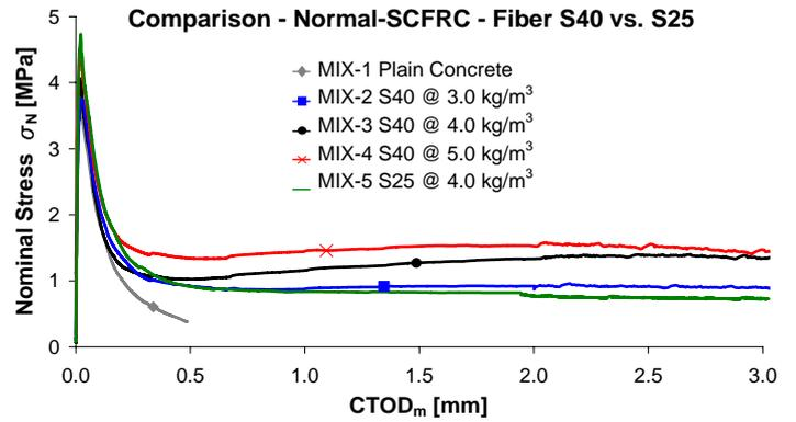
Figure 2. Nominal stress versus CTOD curves (average curves) obtained from bending tests on N-SCFRC specimens.
