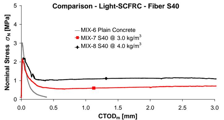
Figure 3. Nominal stress versus CTOD curves (average curves) obtained from bending tests on L-SCFRC specimens.
