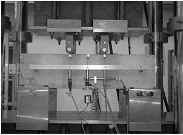
Figure 1. Geometry (a) and instrumentation (b) of the notched specimen for the bending tests, according to UNI 11039.
