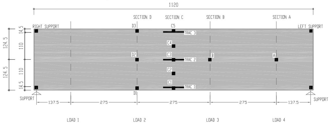
Figure 10. Instrumentation used during the tests.
