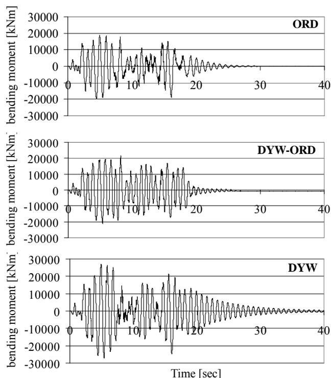
Figure 11. Bending moment versus time for varying critical zone typologies.
