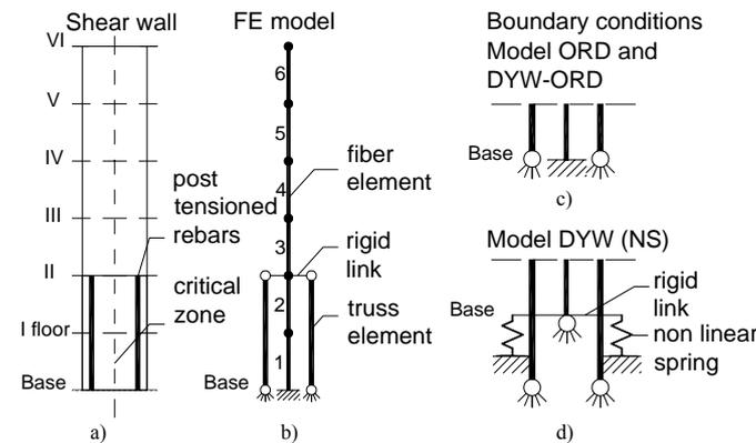
Fig 1. Model A – Force based fiber element mesh.
