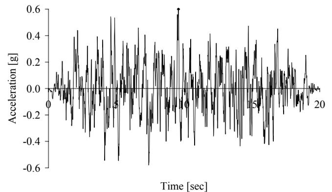
Fig. 7. Adopted EC8 compatible earthquake.
