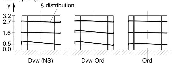
Figure 12. Strain distribution in reinforcement and concrete at different wall heights in case of maximum displacement.
