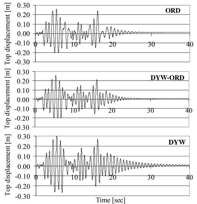
Figure 9. Top displacement versus time for varying critical zone typologies.
