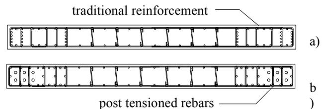
Figure 4. Typical critic zone cross section for: a) traditional walls; b) reinforced shear wall with post-tensioned rebars.
