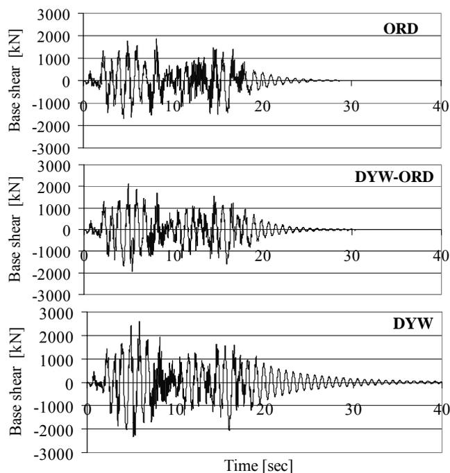
Figure 10. Base shear force versus time for varying critical zone typologies.
