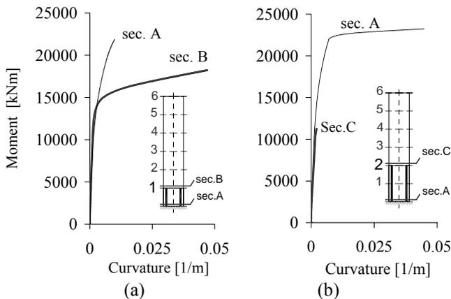
Figure 6. Moment vs curvature for DYW-ORD\_6d32 models as a function of the post compressed zone length.
