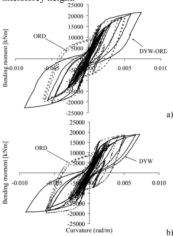
Figure 8. Moment versus base rotation curve for: (a) ORD and DYW-ORD; (b) ORD and DYW models.
