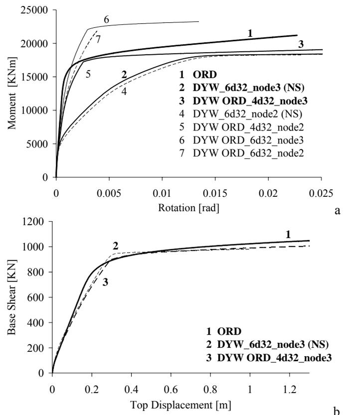
Figure 5. Pushover test: a) bending moment versus base section rotation; b) Base shear versus top displacement.
