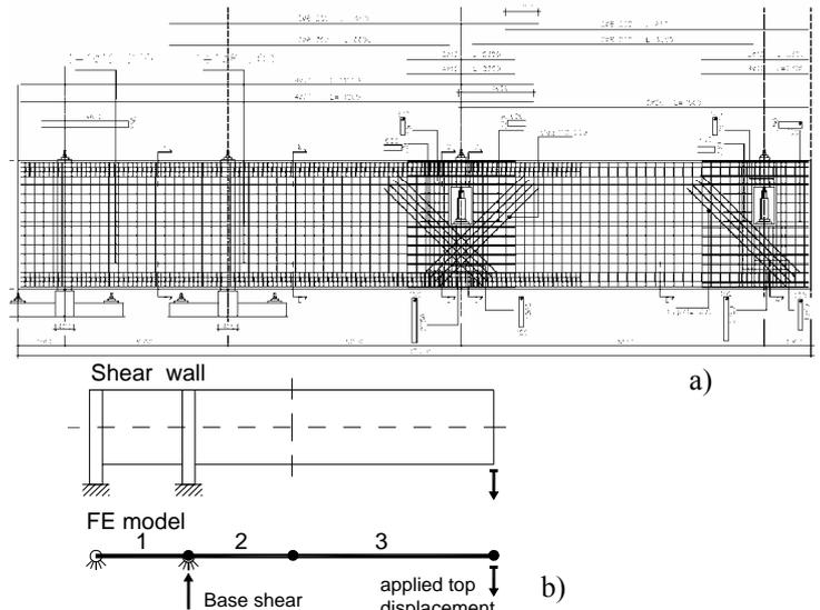
Figure 2. (a) Experimental 1:1 scale R.C. wall (Riva e al. 2000) and (b) numeric model.
