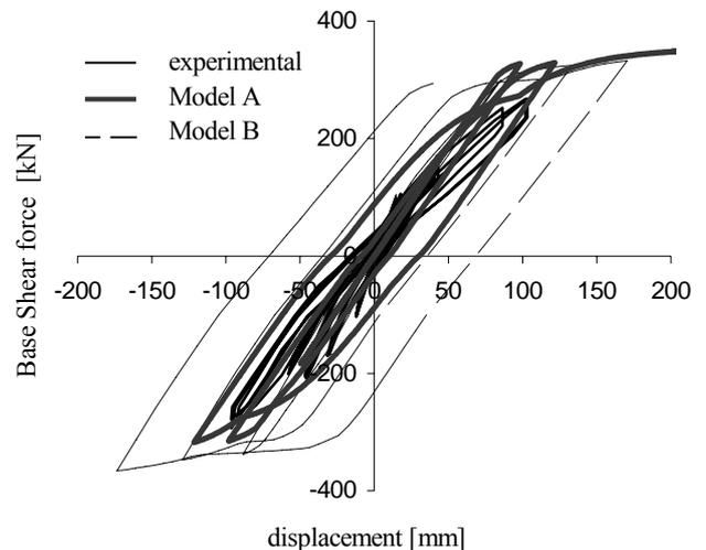
Figure 3. Numerical and experimental response.
