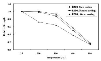
Figure 9. Relative residual strength vs. maximum temperature
