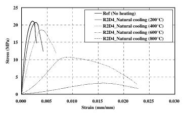
Figure 7. Axial stress-strain response (Natural cooling)
