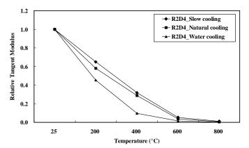
Figure 10. Relative initial tangent modulus vs. maximum temperature
