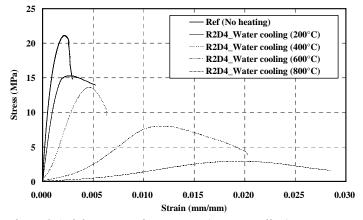
Figure 8.Axial stress-strain response (Water cooling)
