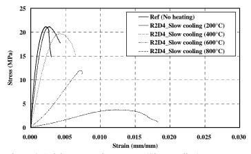
Figure 6. Axial stress-strain response (Slow cooling)
