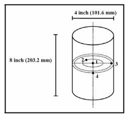
Figure 2. Locations of thermocouples and specimen geometry
