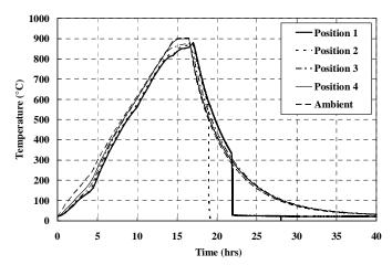
Figure 3. Transient temperature at each position in the concrete cylinder
