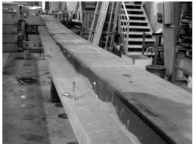
Figure 14: View of Beam P2 after failure.
