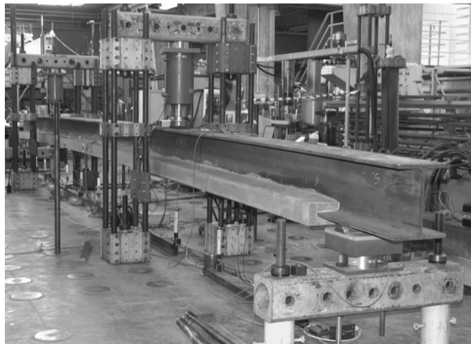
Figure 5. Transfer of prestressing to the composite beam at 48 hours of concrete age.
