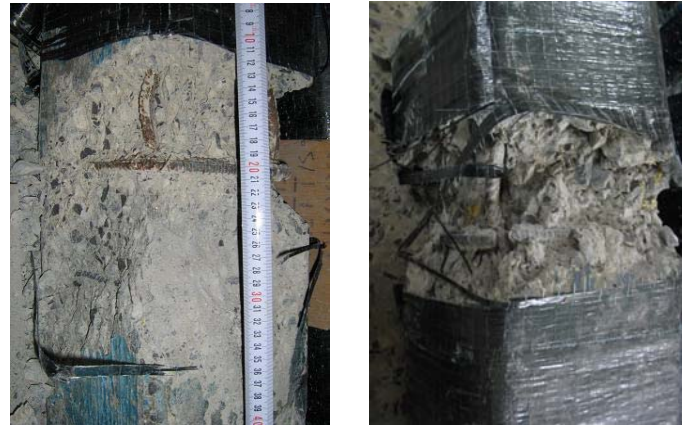
Figure 4. Failure mode for C3L8S8 and C3L4S12
