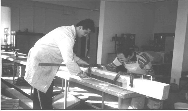
Figure 8. Process of placing the epoxy plates.
