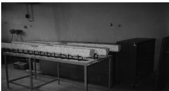
Figure 4. U-shaped stirrup anchoring from underneath.
