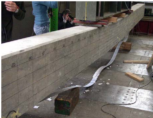
Figure 11. Failure of beam PRC-PrEA.
