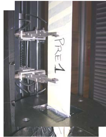
Figure 4. Tensile test on CFRP laminate (configurations before and after the test)
