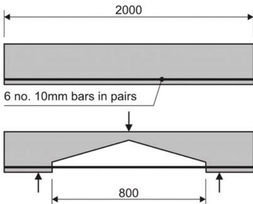
Figure 12. Test beams according to Beeby (2000), showing that removal of a part of the concrete can cause a considerable increase of the bearing capacity.
