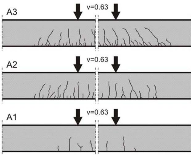
Figure 6. Crack pattern development in shear critical beams ( $a/d = 3$ ), with cross sectional depths varying from 750 mm (beam A<sub>3</sub>) to 150 mm (beam A<sub>1</sub>), represented equally large, at the same nominal shear stress  $V/bd = 0.63$  MPa.
