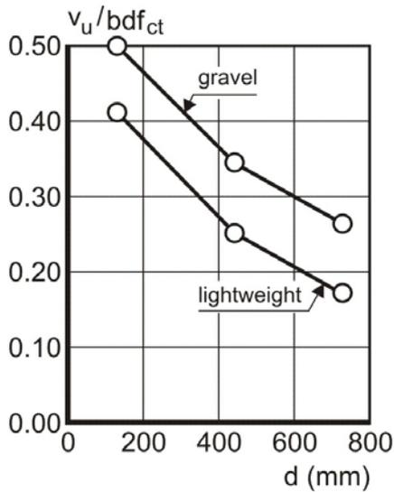
Figure 5. Nominal shear strengths as a function of the effective cross sectional depth, for gravel – and lightweight concrete (Walraven, 1978).
