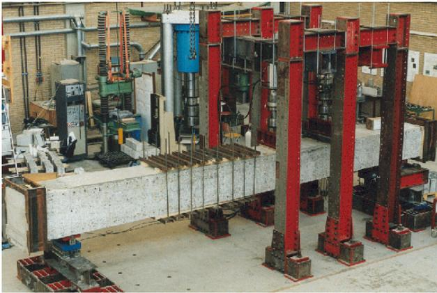
Figure 7. Shear test on strip, sawn out of an existing slab viaduct, with an unusual relation of concrete tensile to concrete compressive strength.
