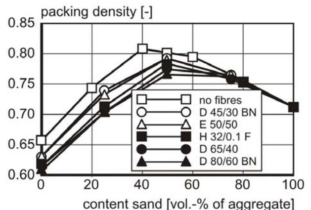
Figure 17. Effect of the sand content and the type of steel fibres (at 1.5 Vol.%) on the packing density (fibre types: first index:  $L_f/d_f$ ; second index:  $L_f$ ), according to Grünwald, 2004.
