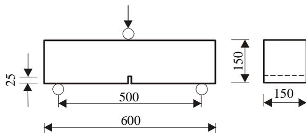
Figure 19. Rilem standard test for fiber concrete.
