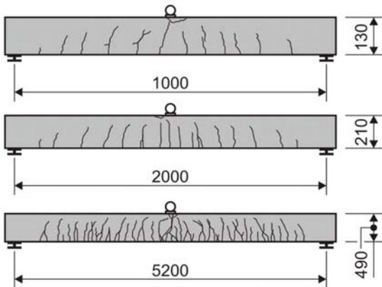
Figure 14. Crack patterns for rotational capacity tests on beams with different depths and a reinforcement ratio of 1.12%, after Bigaj, 1999.
