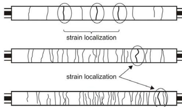
Figure 22. Crack patterns in centrally loaded reinforced tensile bars. From top to bottom 0, 0.8 and 1.6 Vol.% short steel fibers: (Shionaga, 2006)
