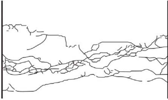
Figure 2. Crack band in a concrete with  $d_{\max} = 16\text{mm}$  (van Mier, 1996).
