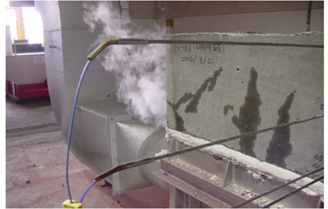
Figure 17. Vapor eruption from cracks of the specimen.
