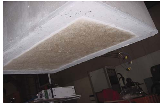
Figure 41. Surface of fire protection coating after test.
