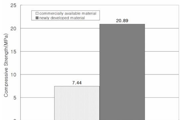
Figure 1. Comparison of compressive strength of commercially available material and new material.
