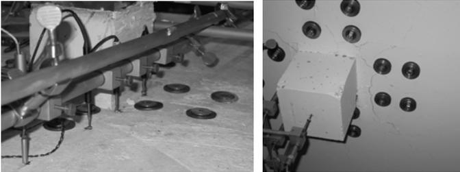
Figure 1. Strengthened slab with shear-bolts.
