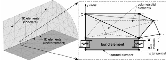
Figure 4. Definition of the bond element.
