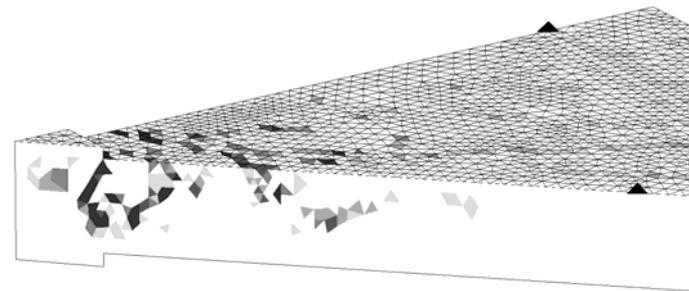
b) Tensile strains in x-direction - flexural cracks
