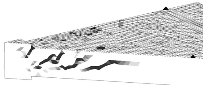
c) Tensile strains in z-direction – shear cracks
