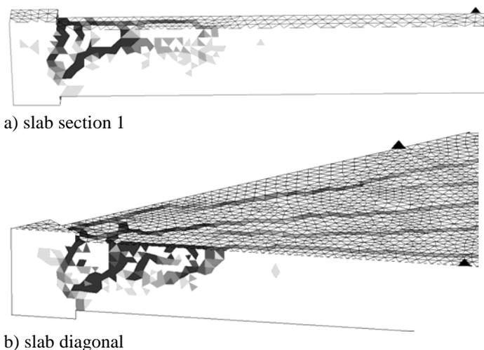
Figure 9. Cracking at ultimate load: SB1.
