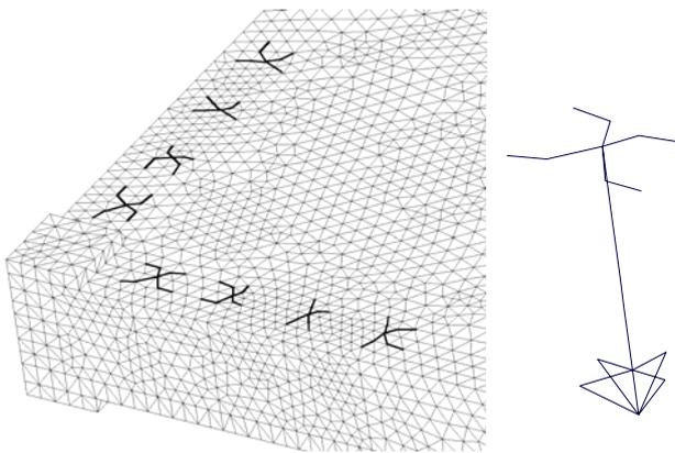
a) Slab section with column stub
