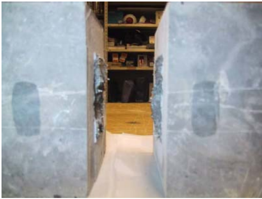
Fig. 17 Typical fracture in Series 3.
