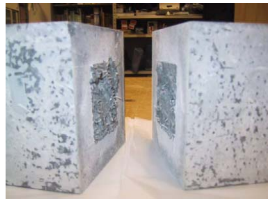
Fig. 14 Typical fracture in Series 2.
