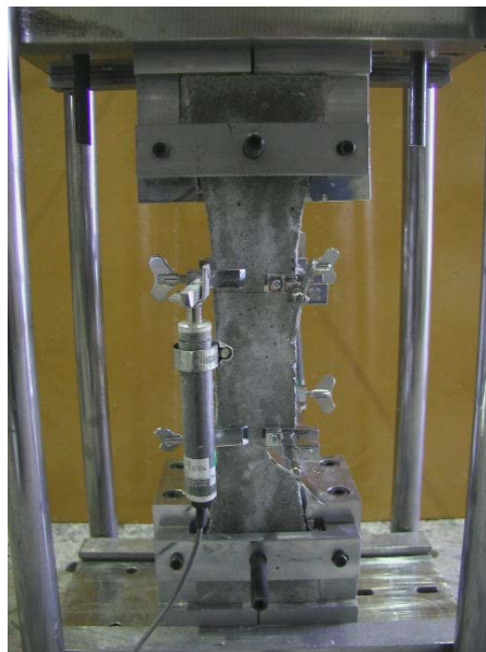
Figure 2. Uniaxial tension test setup.
