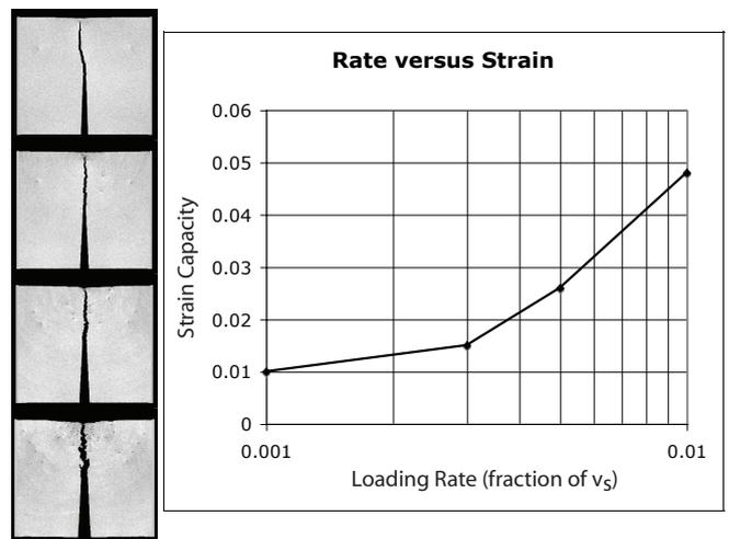
Figure 3. Crack propagation profile represented in density variation. Specimens corresponding to near separation configurations (From the top, loading rates are 0.1%, 0.3%, 0.5%, 1.0%, and 5.0% of  $v_s$ ). Global strain at each row is 1.0%, 1.5%, 2.6%, and 4.8%.
