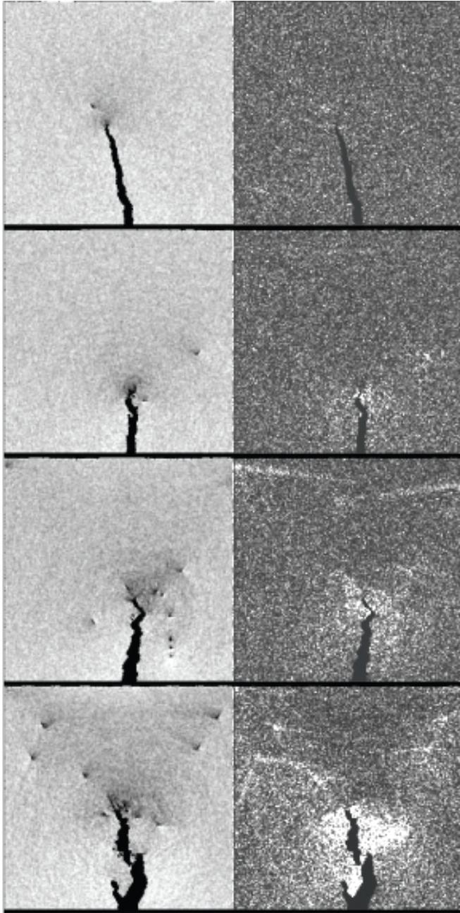
Figure 5. Magnified crack tip corresponding to global strain of 0.33%, 0.50%, 0.86%, and 1.6% from the top (loading rates are 0.1%, 0.3%, 0.5%, and 1.0% of  $v_s$ ). Each snapshot shows the region of  $x \in (185, 415)$  and  $y \in (335, 565)$ . Left column shows density distribution and right column shows temperature distribution.
