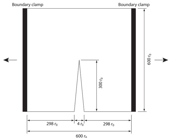
Figure 1. Configuration of the test specimen. Dimensions are in particle units, and 10 layers of boundary particles are padded on both left and right sides to simulate clamps.
