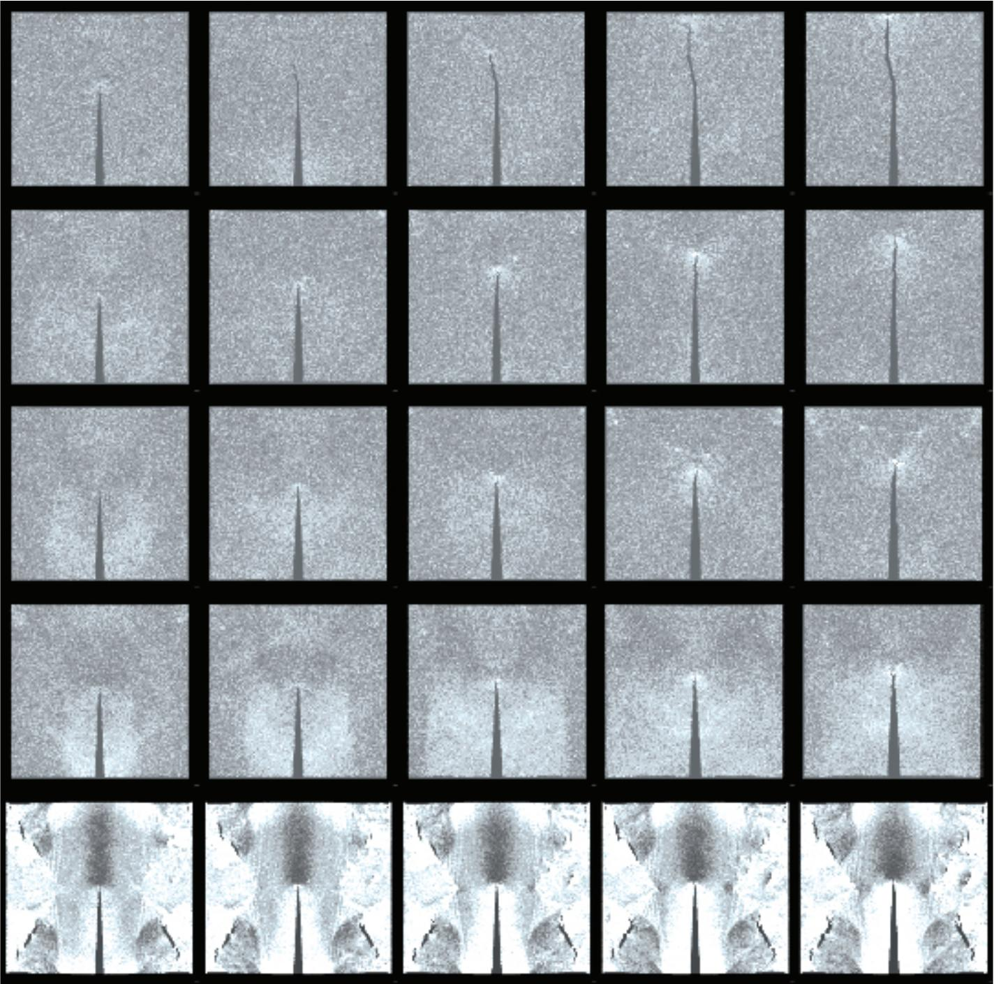
Figure 4. Crack propagation profile represented in temperature variation. Specimens corresponding to 5 different loading rates (0.1%, 0.3%, 0.5%, 1.0%, and 5.0% of  $v_s$ ) are arranged in rows, and each column depicts a snapshot at the same global strain (0.15%, 0.3425%, 0.535%, 0.7275%, and 0.92%). Brightness of the figure is byte scaled to 0–30% of melting point.
