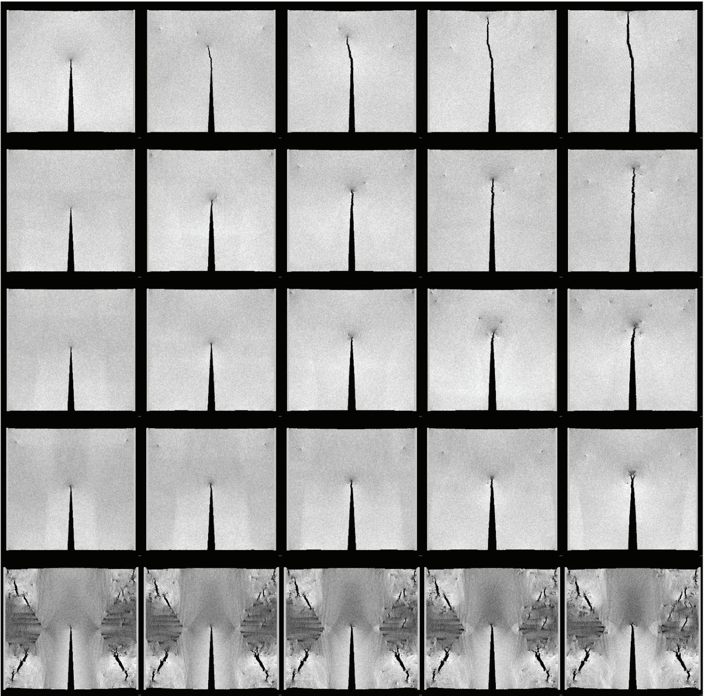
Figure 2. Crack propagation profile represented in density variation. Specimens corresponding to 5 different loading rates (0.1%, 0.3%, 0.5%, 1.0%, and 5.0% of  $v_s$ ) are arranged in rows, and each column depicts a snapshot at the same global strain (0.15%, 0.3425%, 0.535%, 0.7275%, and 0.92%). Brightness of the figure is byte scaled to number density of 1.0–1.2.
