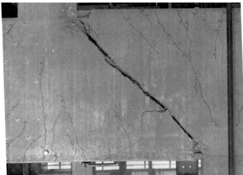
Figure 6: Shear wall tested in the laboratory, Asin (1999).
