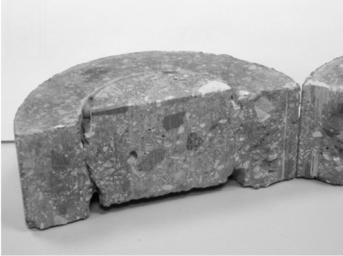
Figure 11. Fracture plane observed in tested specimen.
