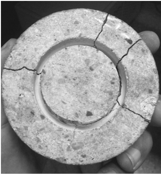
Figure 8. Conventional concrete specimen after the unconfined test, with a total of four large radial cracks and a smaller fifth one in the lower part of the image.
