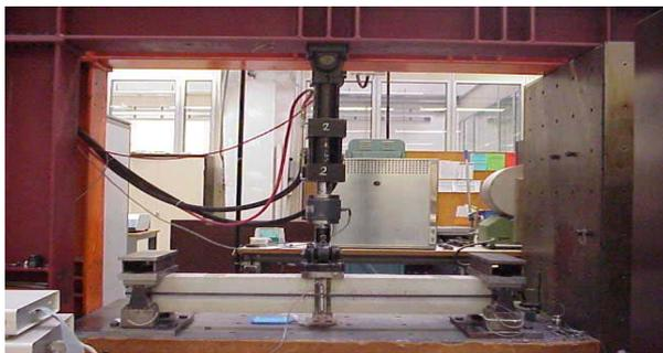
Figure 7. Experimental set-up for cyclic three points bend tests on RC beams.
