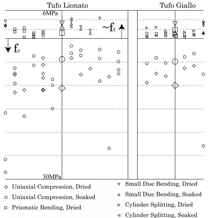
Figure 3. Strength data for Tufo Lionato and Tufo Giallo della Via Tiberina. Each column corresponds to a different quarry. Large markers represent the mean for each type of test result. After De Casa *et al.* (1999, 2007) and Jackson *et al.* (2005).
