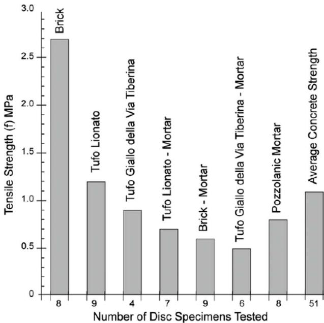
Figure 6. Tensile strengths of components from the wall concrete of the Great Hall, as measured by point source tests.
