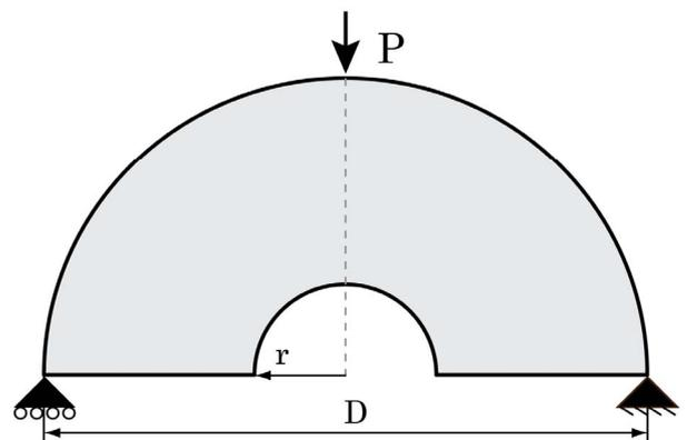
Figure 8. Top: photograph of wall concrete core with components outlined: 1-pozzolanic mortar; 2-Tufo Giallo della Via Tiberina; 3-brick fragment; 4-Tufo Lionato. The outer core diameter is 20cm. Bottom: schematic of test design.  $D = 20\text{cm}$ ;  $r = 5\text{cm}$ .
