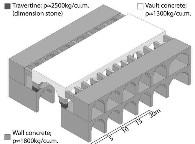
Figure 2. Computational solid model of the Great Hall, showing the three structural-scale materials.
