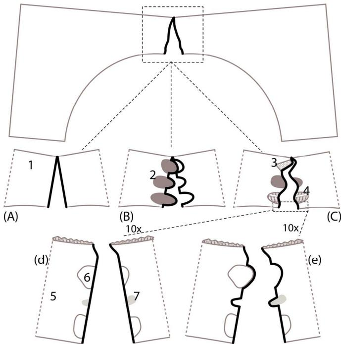
Figure 7. Schematic showing possible meso-scale (A-C) and micro-scale (d-e) mechanisms of fracture in a Roman concrete vault.
