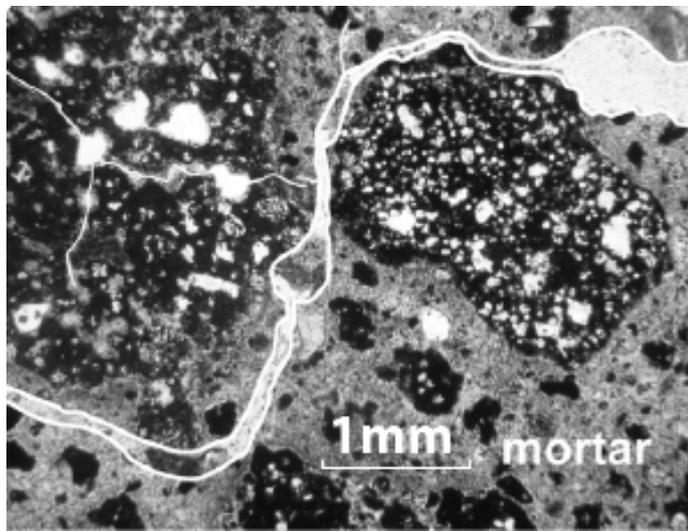
Figure 4. Photomicrograph of the curving trajectory of a debonding crack that follows the perimeters of Pozzolane Rosse scoriae in a mortar sample from the Great Hall, produced by a point source load test (after Jackson *et al.* 2009).
